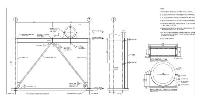
Figure 1 – Temporary Support Cradle and Frame
